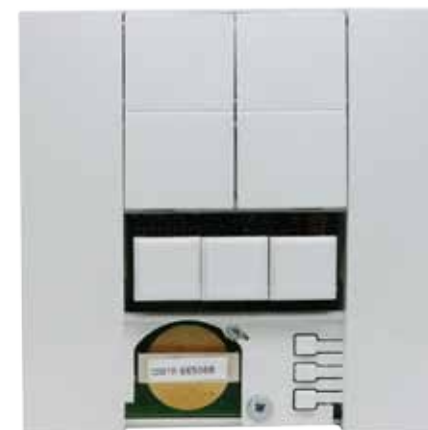
Cover lifts off for programming
