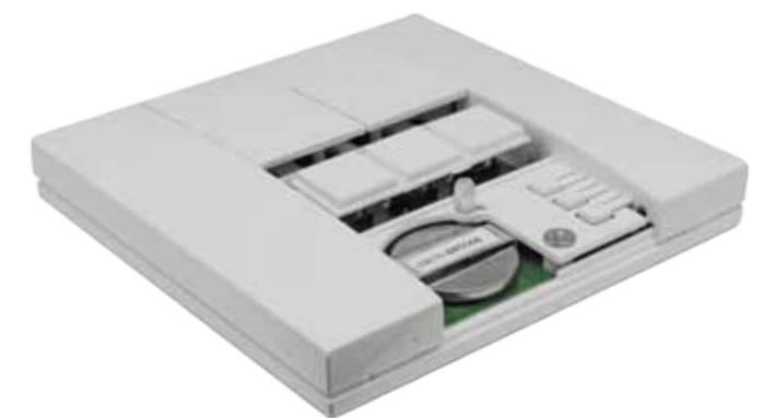
Battery slots in here
