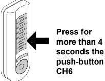
1- Press and hold down the automatic cycle push button Ch6 for more than 4 sec., the light will turn off and return on once and a second time after 4 sec. which indicates that you have entered
