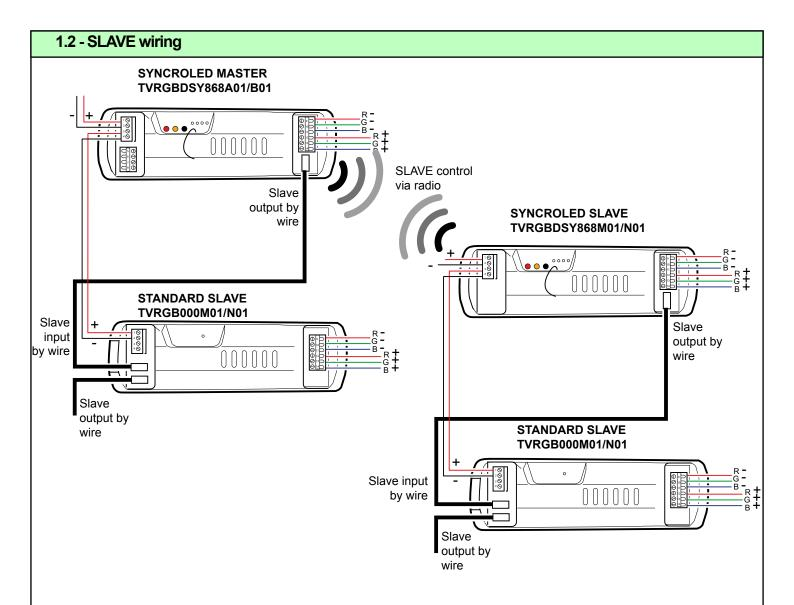
In the field of action of a syncroled system (master+slave) it is not allowed the presence of other system syncroled (master+slave)
