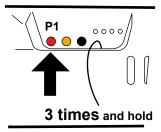
1- Press the push button **P1** three time and hold it down, the buzzer will make a beep each time and then sound slowly and intermittently.
