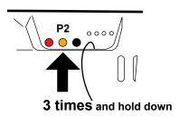
1- Press the push button **P2 three times and hold** it down, the buzzer will make a beep each time and then sound continuously.
