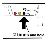
1- Press the push button P3 two time and hold it down. the buzzer will make a beep each time and then sound slowly and intermittently.
