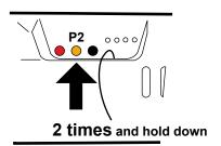
1- Press the push button **P2 twice and hold** it down, the buzzer will make a beep each time and then sound continuously.
