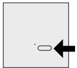
2- Hold down the push button for 10 sec., after this 10 sec. the buzzer will sound continuously by indicating that the whole memory has been cancelled.
