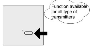
3- During the sound press the push-button of the **new transmitter** which has to be memorised; the memorization is indicated by the intermittently sound of the buzzer.
