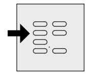
2- During the sound press the push button of the transmitter which has to be memorised, the memorization is indicated by the intermittently sound of the buzzer.
