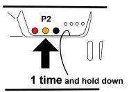
1- Press the push button **P2** once and hold it down, the buzzer will make a beep and then sound continuously.
