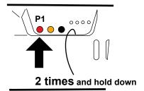
1- Press the push button P1 twice and hold it down, the buzzer will make a beep each time and then sound continuously.
