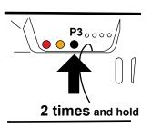
1- Press the push button **P3 two time and hold** it down, the buzzer will make a beep each time and then sound slowly and intermittently.
