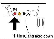
1- Press the push button **P1 once and hold** it down, the buzzer will make a beep each time and then sound continuously.
