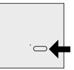
2- Within 5 seconds press a push-button of the **already memorized transmitter** from which the function has to be copied. The buzzer will interrupt the sound for 1 sec., and then carry on for 5 seconds.
