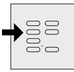
2- During the sound press the push button of the transmitter which has to be memorised, the memorization is indicated by the intermittently sound of the buzzer. All the 4 push-buttons of the transmitter are automatically memorized.
