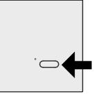
2- During the sound press the push-button which has to be deleted; the deletion is indicated by the continuously sound of the buzzer.
