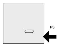
1- Press the button **P3** located inside the **already memorized transmitter**. The enabled receiver sound continuously.
