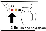
1- Press the push button **P1 twice and hold** it down, the buzzer will make a beep each time and then sound continuously.
