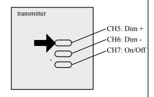
3- Press the push-button which has to be memorised; the memorization is indicated by the quick flash of the led 1.
