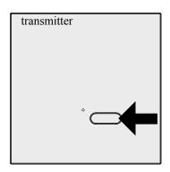
3- Press the push-button which has to be memorised; the memorization is indicated by the quick flash of the led 1.
