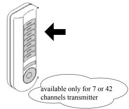
3- Press one push button, of the 7-channel transmitter which has to be memorised, the memorization is indicated by the quick flash of the led 1.
