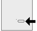
2- Within 5 seconds press a push button of the **already memorized transmitter** which has to be copy the function. Led 1 turns off for 1 sec, and then it turns on for 5 seconds.
