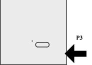
1- Press the button **P3** located inside the **already memorized transmitter**. Led 1 turns on. (the push button P3 is locate inside the transmitter, see transmitter manual)
