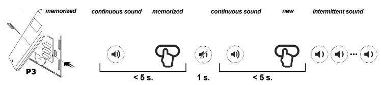
Press the button **P3** of the **memorized** transmitter. Press the button relative to a **memorized** code. Press the button relative to the **new** code.
