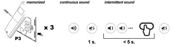
Press three times the button P3 of the memorized transmitter. Press the button relative to the code to delete.
