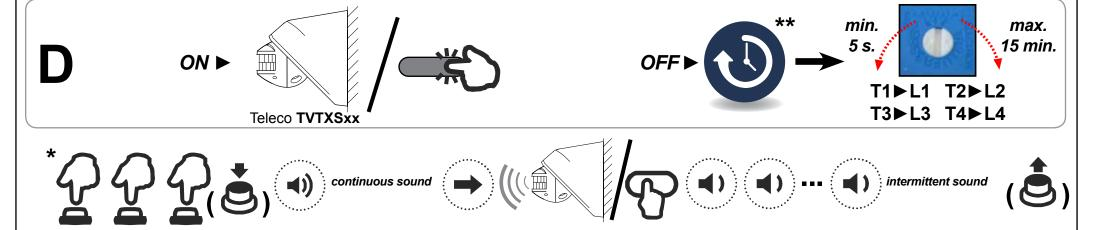
Press 3 times the button relative to the output (M1..M4) and keep it pressed. Press the button of the transmitter relative to the code to memorize or activate the sensor.
