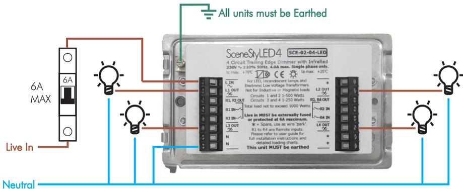
The cable connected to the Live-in terminal must be capable of supplying the total current for all circuits and be protected by an external fuse or circuit breaker rated at 6A maximum.
