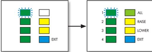
*This shows every circuit being adjusted equally in scene 1.*
