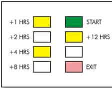
In this example, the +1 HRS, +4 HRS and +12 HRS buttons have all been selected. Therefore, the total time delay is +17 HRS. If the current time was 1:00am, the first step of holiday mode would begin at 6:00 pm that evening. Subsequently, step 2 would start at 6:30pm, step 3 at 7:30pm and so on. The cycle would begin again at 6:00pm the following day.
