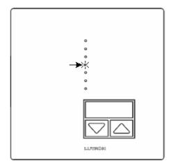
3- Release the Raise button, and after at least one second press and hold it again until the fifth LED begins to flash. The fifthe LED flashing indicates Advanced Features Menu
