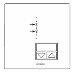
9- Press and hold the Toggle button until all the LEDs stop flashing.
