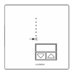
2- Press the Raise button four times, until the fourth LED from the bottom starts flashing.
