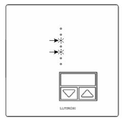
6- Press the Toggle button once. The bottom LED will start flashing rapidly (faster than seen before). This is ELV fine tuning mode.
