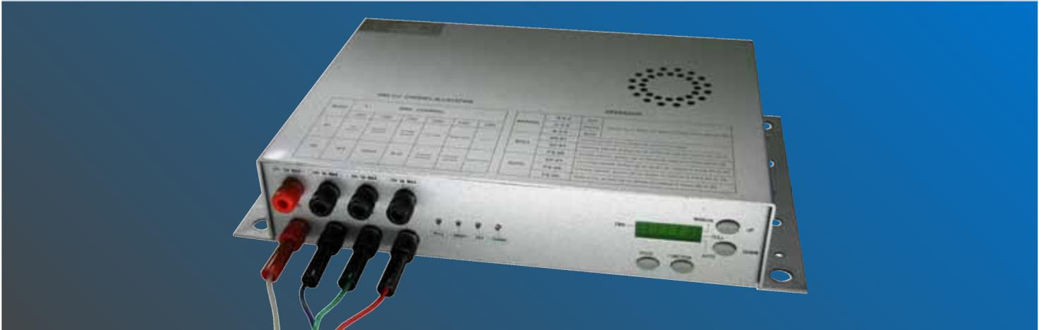
The SRC-171 is a programmable controller for the LED strip above. It is simple to use, but is a very effective tool. This controller has colour mixing programs that are all adjustable. These include colour, speed and strobe programs. This control can be interfaced with Lutron or Rako control systems.
