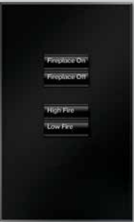
Contact-closure control with seeTouch buttons.
