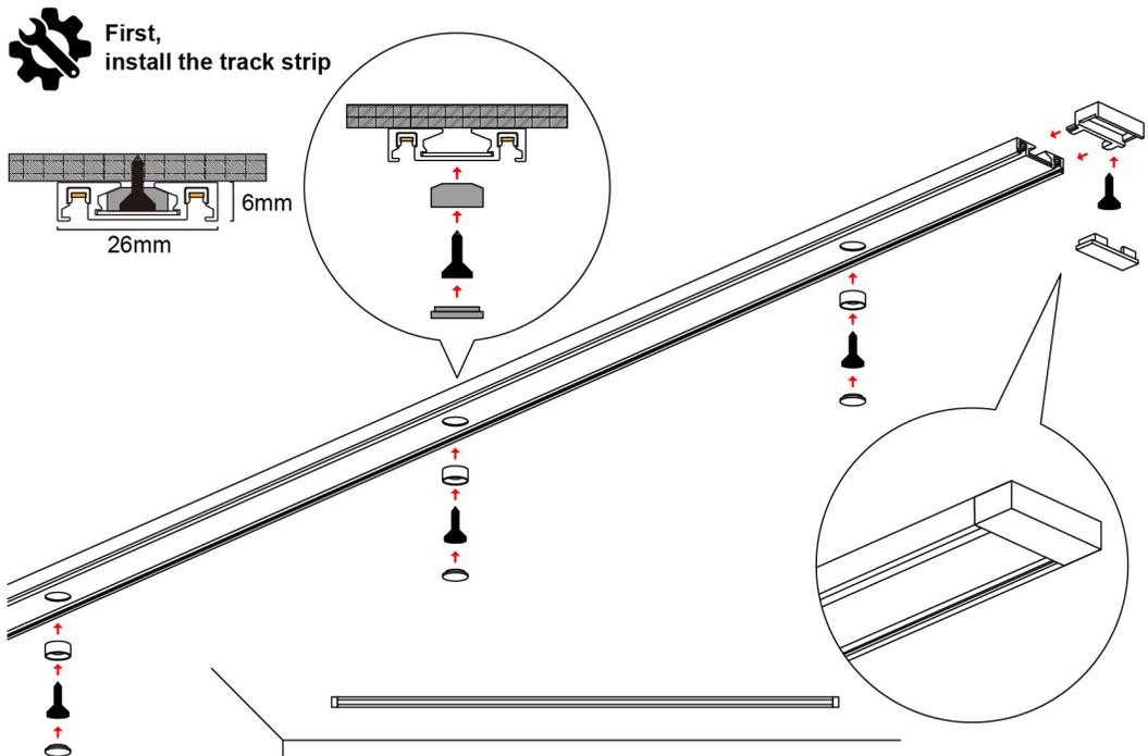
1. Check the fittings: Ultra-thin track strip + Positioning plug + Screws + Screw hole cover
