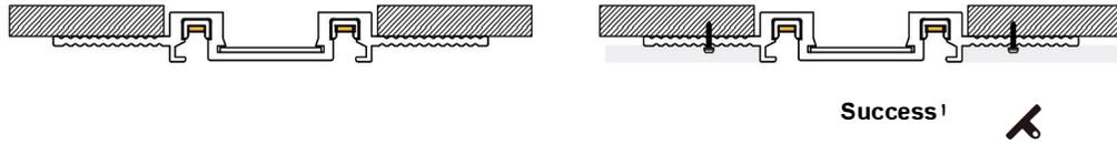
2. Adjust the rail bar clamp plate, use the self-tapping screw to fix,
