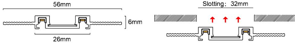
1. According to the section size of the track and the required shape, make the corresponding width of the wood-working plate groove in the ceiling (the strength of the groove body to withstand the weight of the track and lamps, the height of the groove body should be guaranteed in the loading track)
