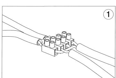
Fit the conductors in the terminal block.
