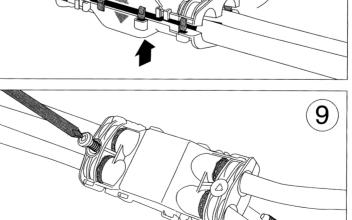
Lock the box tightening the screws.
