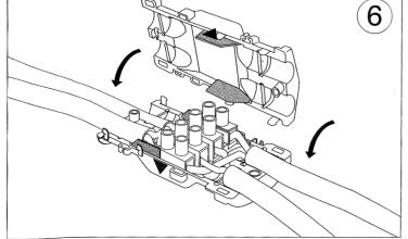
To re-open the box unscrew the screws and unfasten the hooks by screwdriver.
