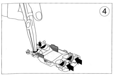
Break the pre-cracked membranes according to cables entry.
