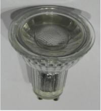
The GU10 LED 6W is a 5W LED lamp designed to fit in any GU10 lampholder. The GU10 LED 5W is fully dimmable with all leading edge dimmers (we recommend against trailing edge) and also complies with the April 2013 Part L Regulations.
