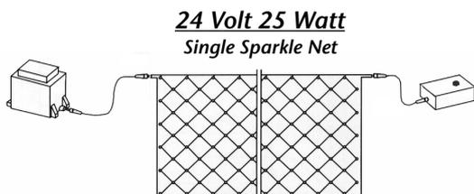
**SINGLE SPARKLE NET 24v 25w 84 lamp indoor/outdoor string complete with a transformer and a chase controller**
