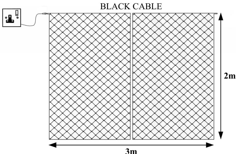
**GIANT SPARKLE NET 240V 480 lamp outdoor waterproof rubber net complete with a 13 amp plugtop**
