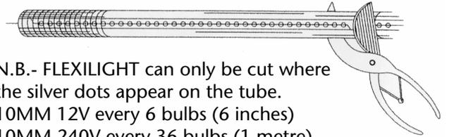
N.B.- FLEXILIGHT can only be cut where the silver dots appear on the tube.
