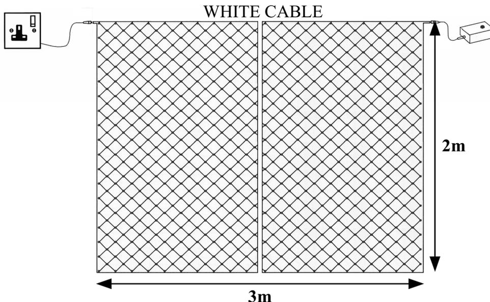
**GIANT SPARKLE NET 240V 480 lamp indoor net complete with a chase controller and a 13 amp plugtop**
