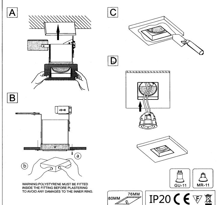
Only fix fixing arm when the lagging is above the fitting. It must be extended to it's maximum height.
