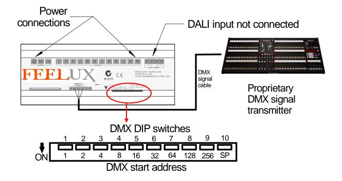
The DIP switches are coded for binary number setting. The start address may be set from 1-508.
