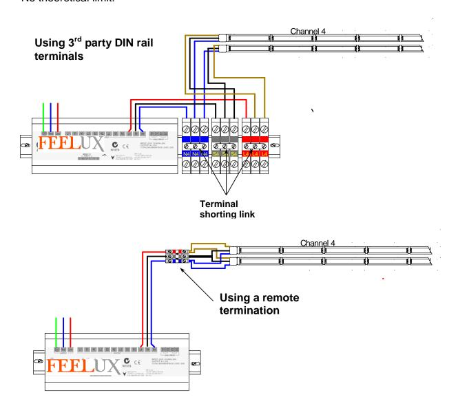
Alternative connection for multiple DimSlim Bus Lines – using remote and/or linked terminals. There is no theoretical restriction to the length of cable or position at which the termination is made.
