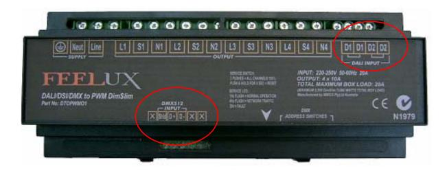
For pin connection onto a DMX circuit, the pin out code is: D+ (plus) XLR pin 3, D – (minus) XLR pin 2, shield (ground) XLR pin 1
