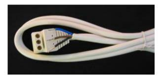
connector's cable has 3 conductors: Brown - Live, Blue - Neutral, Black - PWM signal. Any standard power cable capable of handling the power requirements of the DimSlim fixtures can be used between the DimSlim fixtures and the PWM translator.
