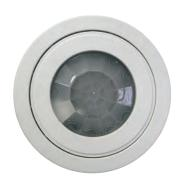
Ceiling flush-mounted PIR occupancy switch with daylight linked dimming. Bring lights on only when area is occupied. Automatically dim lights according to ambient light level, to maintain constant brightness of between 100 and 1000 lux (adjustable). Adjustable time lag before switching off. For suspended or plaster-board ceilings.
