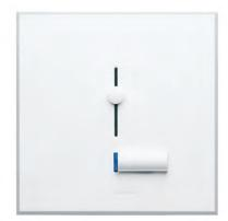
The Lutron Lyneo LNTV-F20BFAWM is a 0-10V dimmer. It needs to be used in conjunction with a 1-10V Interface and will allow up to 20 DimLine fittings to be controlled.
