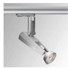
Pixo Pro XS Cool 50 is a slim spotlight for low voltage QR-CB51 lamps. Pixo Pro XS is made of polycarbonate and PPS. Available in white and silver colour. To be used on ceiling or wall mounted tracks (Nanotrack LS1 or Microtrack LS3). Adjustability: turn 0 –  $360^{\circ}$ , tilt 0 –  $90^{\circ}$ . Pixo Pro XS is supplied inclusive glare shield. Integral electronic transformer, dimmable with dimmers that are suitable for electronic transformers.
