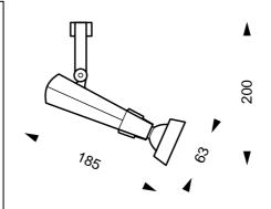
Monopoints allow adapter spotlights to be surface mounted to ceiling or wall. Cover up terminal boxes completely.
