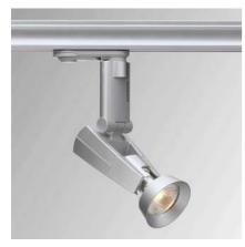
Pixo Pro XS Hi-Spot ES50 is a slim spotlight for mains voltage QPAR51 lamps (Sylvania Hi-Spot ES50). Pixo Pro XS is made of polycarbonate and PPS. Available in white and silver colour. To be used on ceiling or wall mounted tracks (Nanotrack LS1 or Microtrack LS3). Adjustability: turn  $0 - 360^{\circ}$ , tilt  $0 - 90^{\circ}$ . Dimmable with any dimmer. Pixo Pro XS is supplied inclusive lamp and glare shield.
