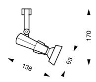
Monopoints allow adapter spotlights to be surface mounted to ceiling or wall. Cover up terminal boxes completely.
