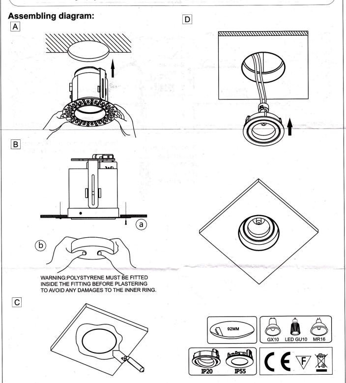
Only fix fixing arm when the lagging is above the fitting. It must be extended to it's maximum height.
