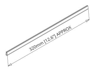
4 - Wrap the rubber cable edge trim around the cable entry/exit holes, making sure the C shape profile is securely pressed all the way around the hole.
