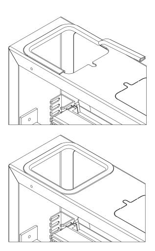
5 - Butt the ends of the edging together for neat finish. Trim off any access length as required.
