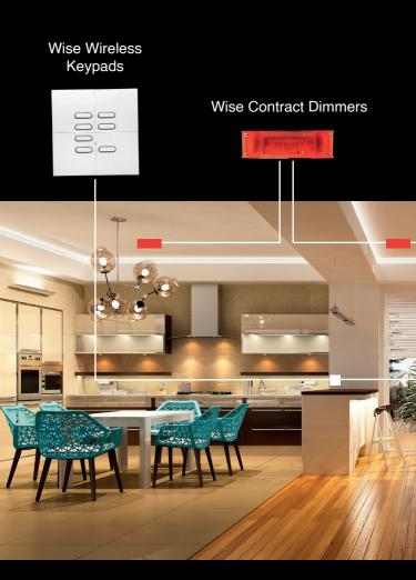
The Wireless Lighting Scene Control System, using wireless, keypads, your phone or smart speaker.
