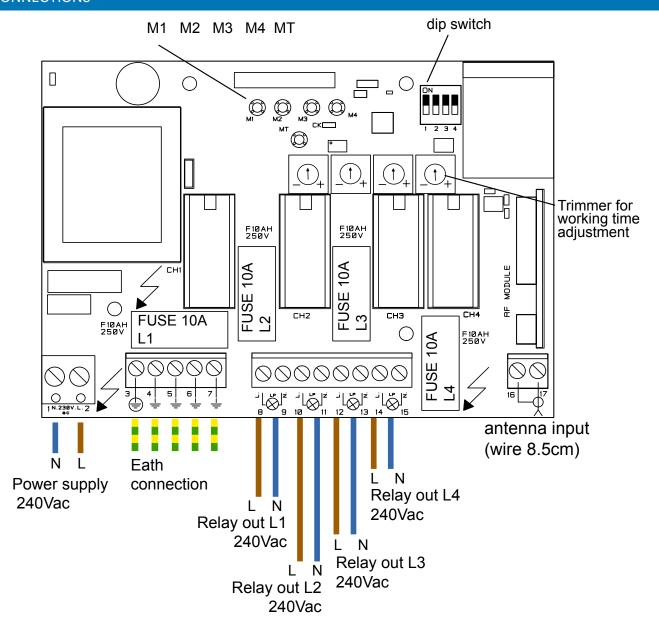
DIP1 - ON L1 Relay with ON/OFF function
