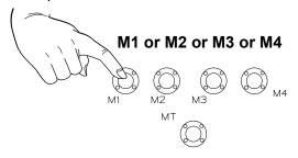
1- Press and hold down one of the push-button **M1 o M2 o M3 o M4** of the receiver, the buzzer will make a beep each time and then sound continuously.
