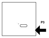
1- Press **three times** the button **P3** placed inside of the transmitter. Buzzer will sound intermittently and slowly.
