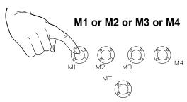
1- Press **twice** and hold down one of the push-button **M1 or M2 or M3 or M4** of the receiver, the buzzer will make a beep each time and then sound continuously.
