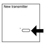
3- During the sound press the push-button of the **new transmitter** which has to be memorised; the memorization is indicated by the intermittently sound of the buzzer.
