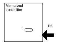
1- Press the button **P3** located inside the **already memorized transmitter**. The enabled receiver sounds continuously.
