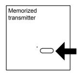
2- Within 5 seconds press a pushbutton of the **already memorized transmitter** from which the function has to be copied. The buzzer will interrupt the sound for 1 sec., and then will carry on for 5 seconds.
