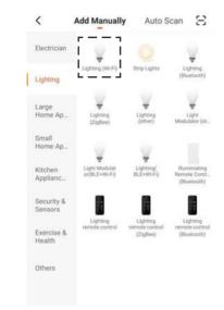
Make sure the Smart Lamp Holder Adapter is fitted correctly, using a suitable Lamp, and then turn the power to the circuit ON. The red Wi-Fi light will automatically flash (if not press and hold the power button located on the front Smart Lamp Holder Adapter for approx. 5 seconds, until the light rapidly flashes). Enter the password for the network and press the 'Next' button.
