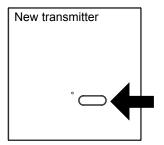
3- During the sound press the push-button of the **new transmitter** which has to be memorised; the memorization is indicated by the intermittently sound of the buzzer.
