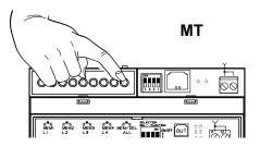
1- Press and hold down the push-button **MT** of the receiver, the buzzer will make a beep each time and then sound continuously.
