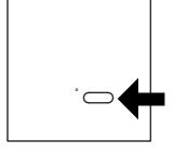
2- During the intermittent sound press the push button which is to be deleted; the deletion is indicated by the continuously sound of the buzzer.
