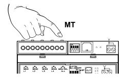
1- Press **three times** the button **MT** and hold down. The buzzer will make a beep each time and then will sound intermittently and rapidly. 2- Hold down the push-button for 10 seconds; after that the buzzer will sound continuously indicating that the memory has been cancelled.
