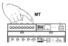
1- Press **twice** and hold down the pushbutton **MT** of the receiver, the buzzer will make a beep each time and then sound intermittently and slowly.
