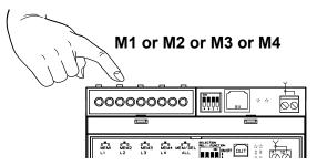
1- Press **twice** and hold down one of the push-button **M1 or M2 or M3 or M4** of the receiver, the buzzer will make a beep each time and then sound continuously.
