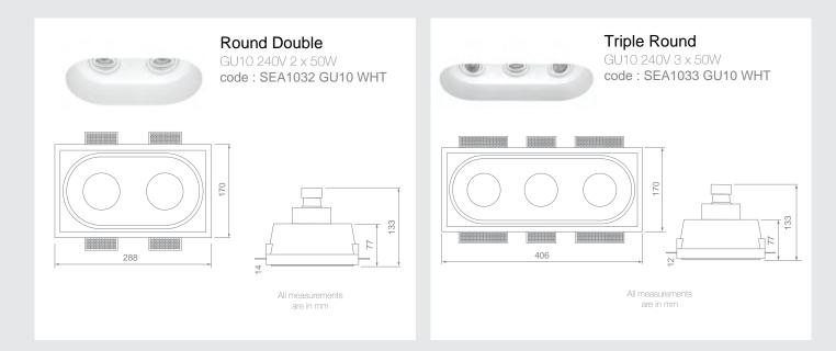
Plaster Downlights are compatible with LED lamps. See www.mrresistor.com for compatible LED Lamps.
