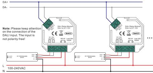
(2) Connecting both Relay & 0/1-10V outputs, switching of 12/24VDC powered 0/1-10V load DALI BUS
