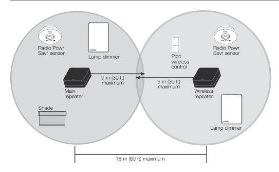
All devices must be located within 9 m (30 ft) of a repeater. The range can be extended with up to four RA2 Select wireless repeaters (Lx-REPPRO).
