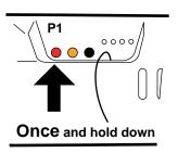
1- Press the push button P1 once and hold it down, the buzzer will make a beep and then sound continuously.
