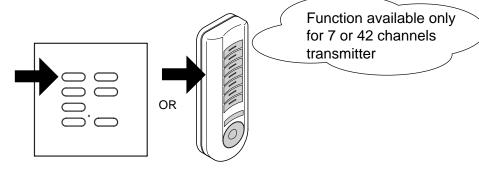
2- During the sound press one push button, of the 7-channel transmitter which has to be memorised, the memorization is indicated by the intermittently sound of the buzzer.
