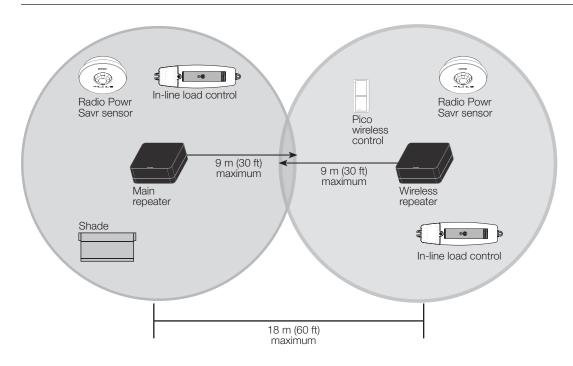
All devices must be located within 9 m (30 ft) of a repeater. The range can be extended with up to four RA2 Select wireless repeaters (LK-REPPRO).
