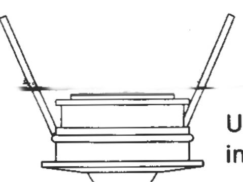
Use this attachment when installing into 50mm plasterboard.
