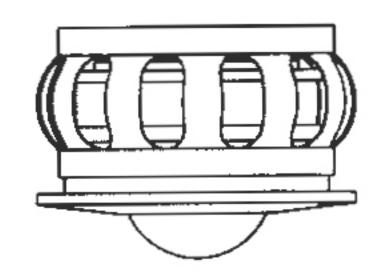
Use this attachment when installing into wood, mdf or 25mm plasterboard.
