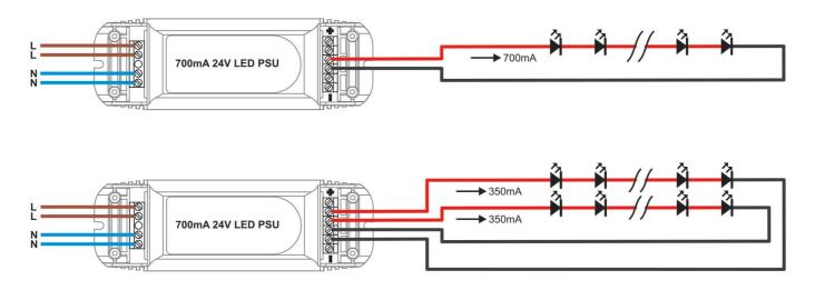
IMPORTANT: Each output MUST drive the same number of LEDs.
