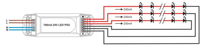
**IMPORTANT:** Each output MUST drive the same number of LEDs.
