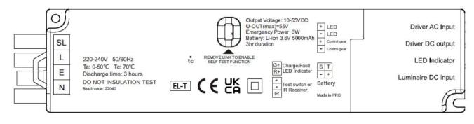
This is a self-test emergency conversion pack. When the self-test system is active, a functional test is carried out automatically once a week and runs for 30seconds. A full duration test is carried out automatically every 52 weeks. The first full duration test is carried out automatically within the first 4 weeks of being connected to mains supply.
