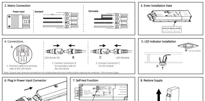
Remove link to enable self-test func on
