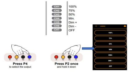
1-Select the output to associate by pressing the button **P4** (the selection will be indicated by the relative led ON). 2- Press the button **P2 once** and hold it down; the buzzer will sound a continuous beep.
