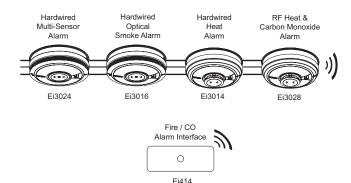
If an Ei3028 Heat and CO Alarm is required on a hardwired section, it should be fitted to a Fire, Smoke and Heat only section, one per section and that Ei3028 should also be the section's link to the RF network of the hybrid system. This ensures that the RF Fire alarm message can be transmitted if any device on the hardwire circuit is activated and the RF CO Alarm message if the Ei3028 detects dangerous levels of CO
